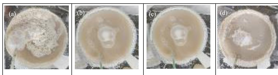
Figure 7. Foaming of diluted FPW aerobic digestion added with biosurfactants after aeration for (a) 30 minutes, 0.04 g RL/g TSS; (b) 2 hours, 0.04 g RL/ g TSS; (c) 30 minutes, 0.15 g SP/g DS; (d) 19 hours, 0.15 g SP/g DS.
